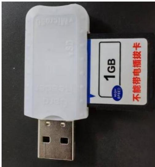
Save the folder to the SD card or U disk and plug it into the USB port of the controller
