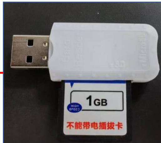
The U disk or SD card is inserted into the USB interface of the controller,
